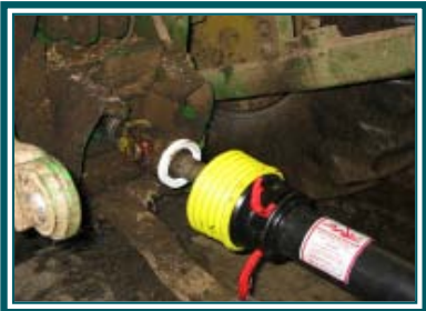
Shield in retracted position for maintenance
