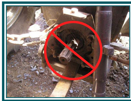
Tractor without the PTO master shield
