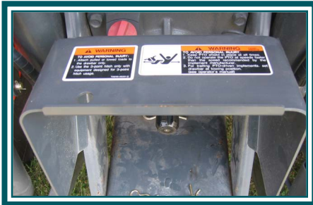
Properly installed tractor master shield covering the PTO stub shaft
