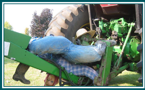
Mock PTO entanglement demonstration
