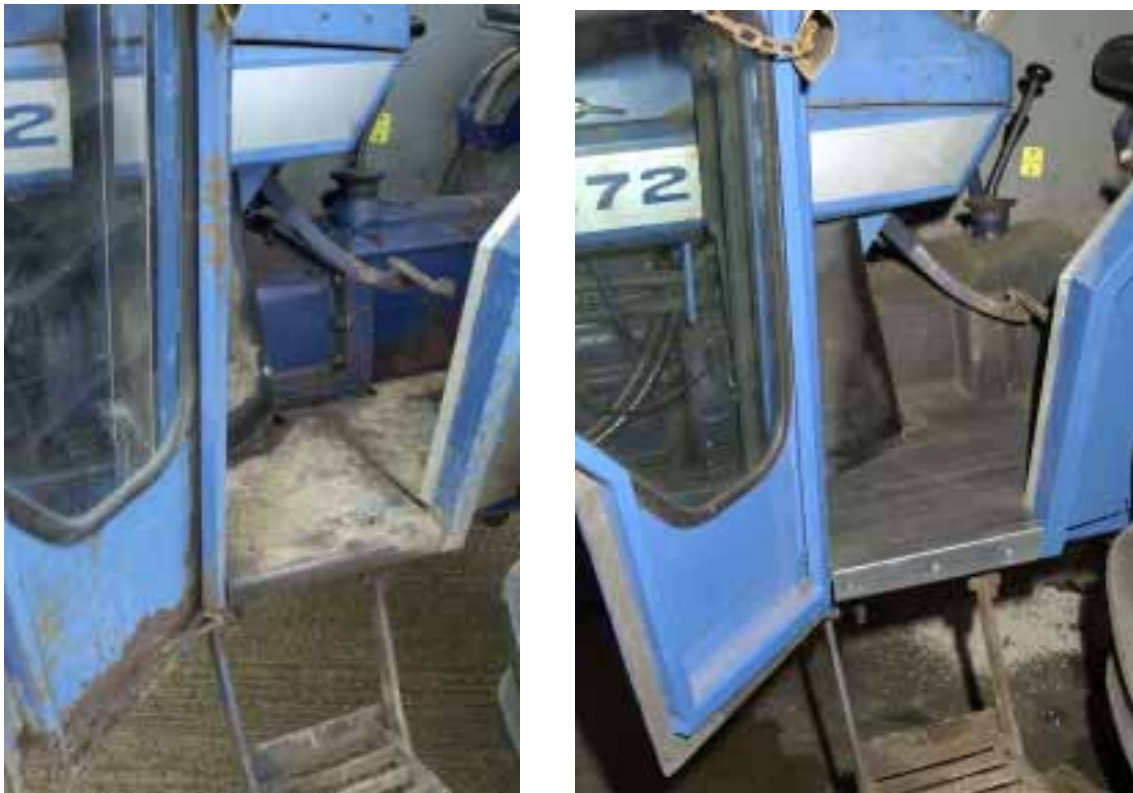
Figure 26 Dilapidated (left) and refurbished (right) tractor Q-cab
