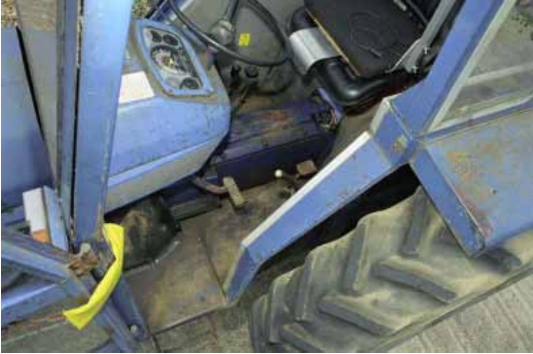
Figure 11 Cab interior showing absence of noise reduction materials
