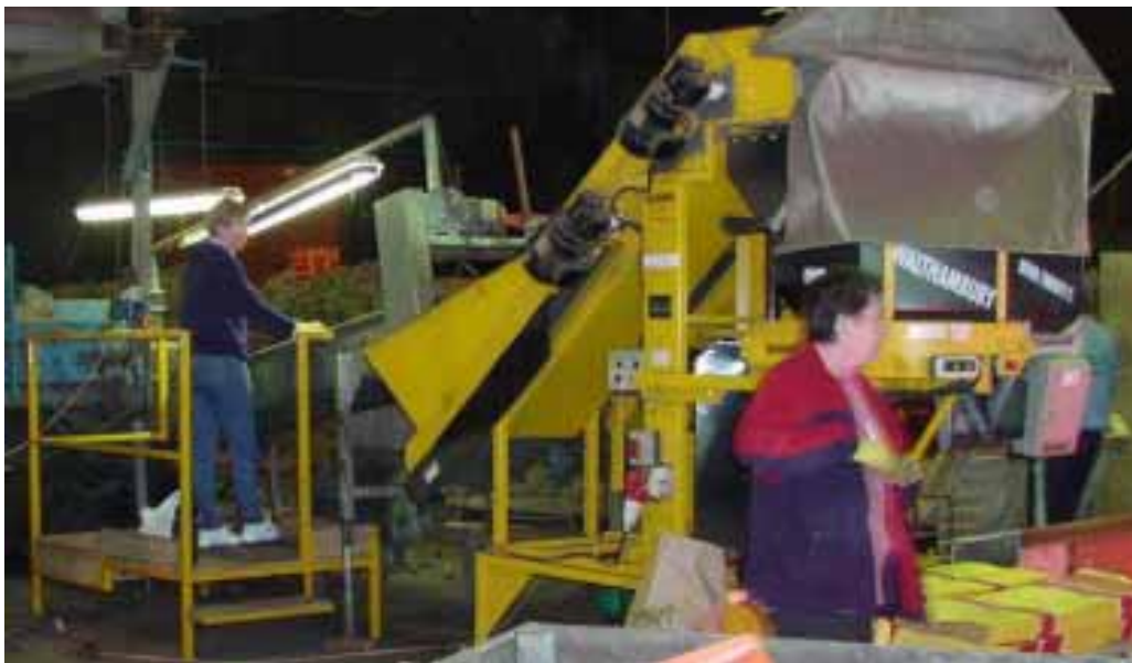
Figure 12 Typical high capacity potato grading and packing line
