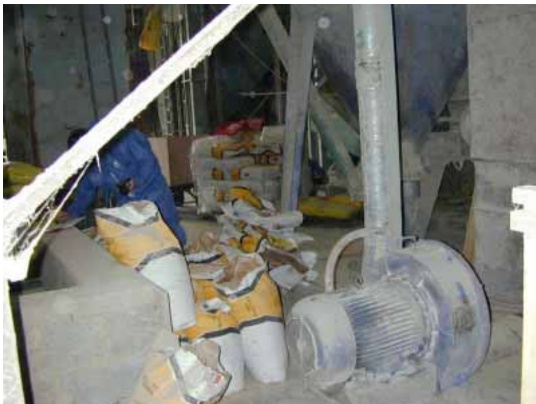
Figure 15 General view of animal feed preparation building with hammer mill shown in the foreground
