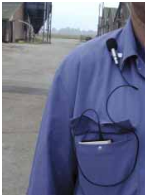
Figure 23 Personal noise dosimeter worn during working period
