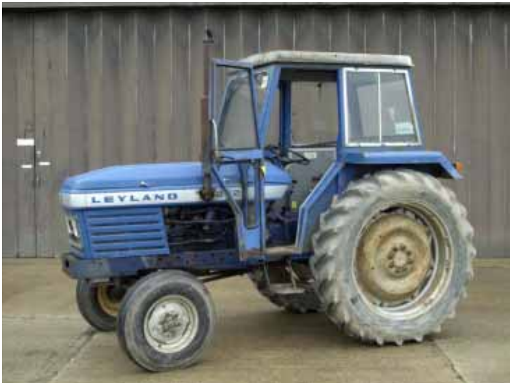
Figure 10 Deteriorated Q-cab on otherwise serviceable 70hp tractor
