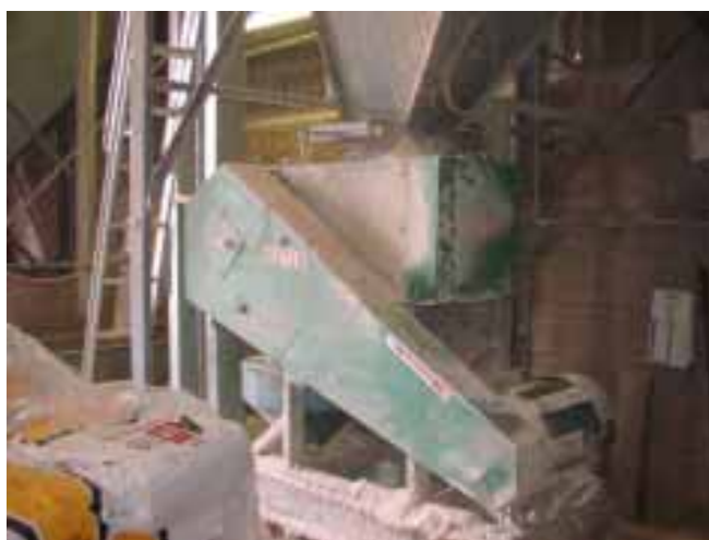
Figure 17 Animal feed cubing machine installation, before (left) and after (right) noise reduction treatment (noise reduction enclosure shown open for machine maintenance)
