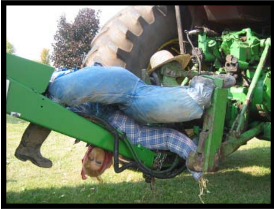
Mock PTO entanglement demonstration
